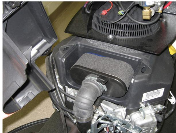
**CAUTION!** Do not wash the air cleaner filters. Do not oil the air filters. Do not use pressurized air to clean the air filters.
