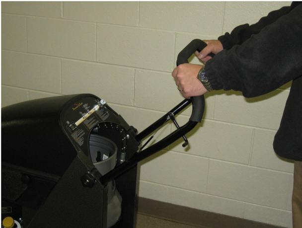
Do not try to start the machine with the bail throttle in the operating position.
