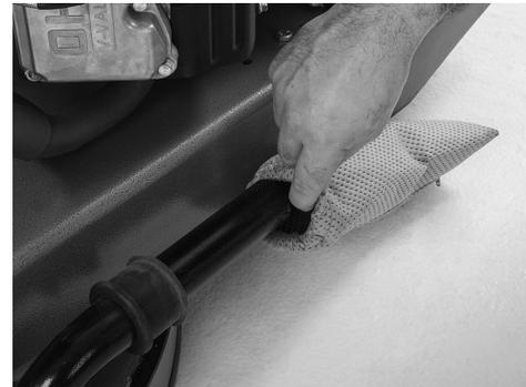
3. Empty bag by rubbing or gently tapping on sides, in a downward motion, to loosen soil trapped on sides of bag. For heavy soil, turn bag inside out to clean.
