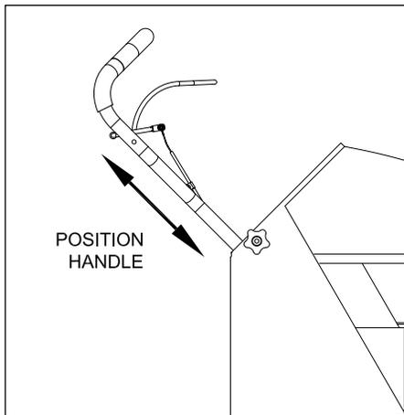
4. Tighten the handle pivotknobs.
