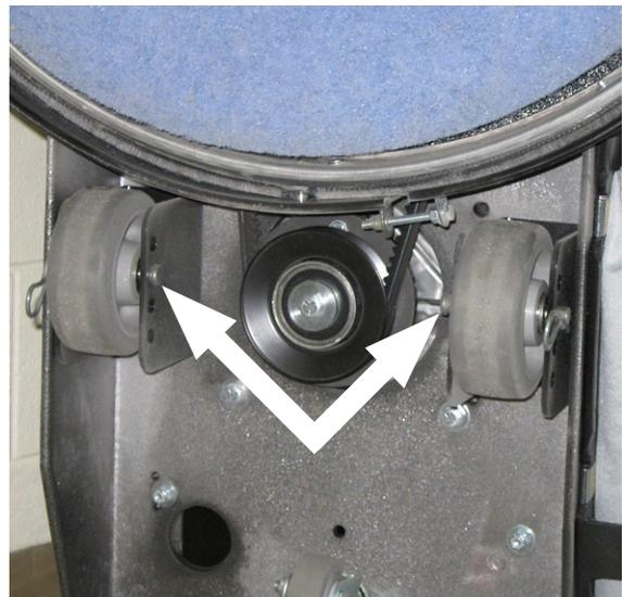
**NOTE:** To increase pad pressure (more aggressive) move wheels to rear of machine. To decrease pad pressure (less aggressive) move wheels toward the front of machine.
