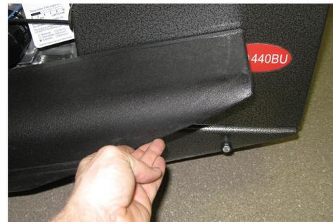
2. Pull the dust bag off the dust tube, keeping the closed end pulled downward to prevent spillage.
