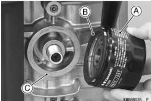
5. Turn the filter until the seal contacts the mounting surface (-C-) of the engine. Then, turn the filter "BY HAND" 3/4 turn more.
