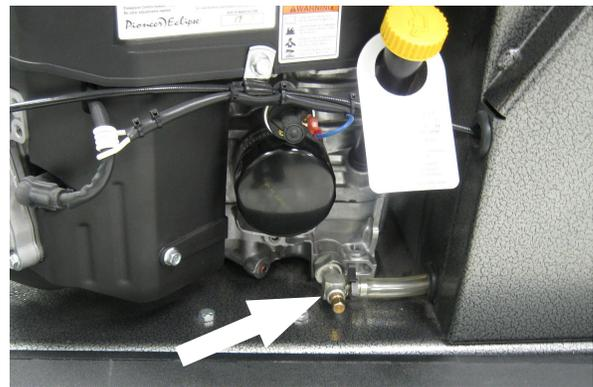
**NOTE:** In order for the oil to drain, it may be necessary to loosen the oil fill cap.
