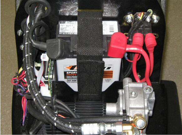
3. Remove the hood that covers the battery and regulator.
