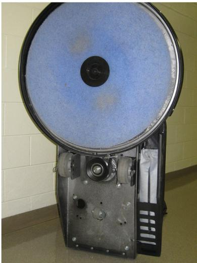
5. Remove centering device and inspect pad. If pad has worn to less than a 1/4" (6mm) thick, replace it.
