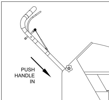
9. Tighten the handle pivot knobs on both sides of the bulkhead.
