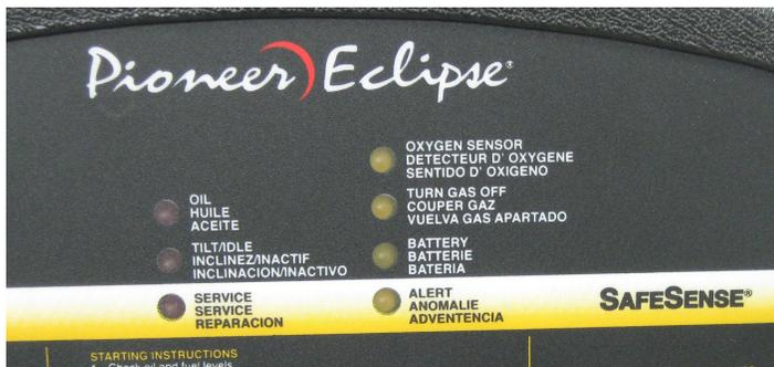
**NOTE:** After engine starts, the **YELLOW** alert light will flash for a 3 minute warm-up cycle of the SafeSense system. (The machine may be operated during this warm-up period.) After the warm-up cycle, the alert light will go out. None of the SafeSense lights will be illuminated as long as the machine is running safely.
