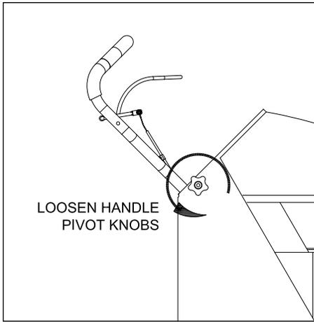
3. Move the handle in and out to the desired height
