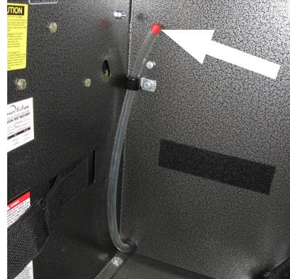
5. Place a suitable container under the end of the oil drain hose.
