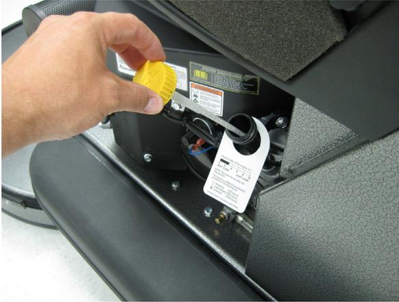
5. The machine should be in an upright level position. If necessary, place a block under the back of the machine or apply weight to the front of the deck to maintain an upright, level position.
